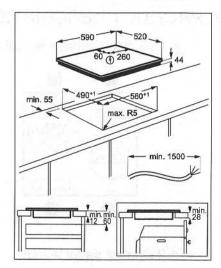
If the appliance is installed above a drawer, the hob ventilation can warm up the items stored in the drawer during the cooking process.
